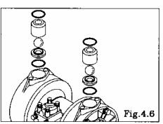
• Remove the O ring, valve stopper, ball and valve seat. [Fig.4.6]
