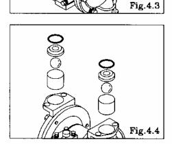
• Remove the O ring, valve seat, ball and valve stopper. [Fig.4.4]
