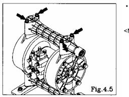
• Remove the 4 retainer nuts from the upper side of tie rods, and remove the out manifold. [Fig.4.5]
