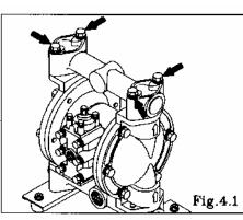
• Remove the 4 retainer bolts from the out manifold, and remove the out manifold. [Fig.4.1]
