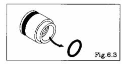
• Remove the packing from the throat bearing. [Fig.6.3]
