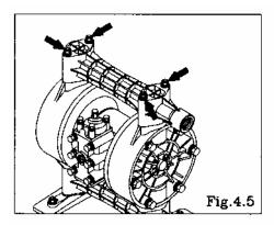
Remove the 4 retainer nuts from the upper side of tie rods, and remove the out manifold. [Fig.4.5]
