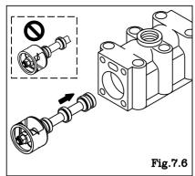
Tightening torque for installation cap A, cap B 4.5 ft-lbf {6 N-m} Tightening torque for valve body installation bolts 5.5 ft-lbf {7.5 N-m}
