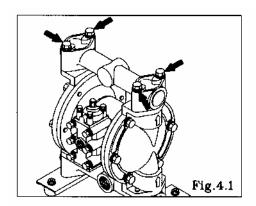
Remove the 4 retainer bolts from the out manifold, and remove the out manifold. [Fig.4.1]
