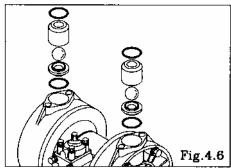
• Remove the O ring, valve stopper, ball and valve seat. [Fig.4.6]
