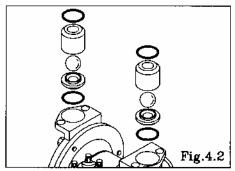
Remove the O ring, valve stopper, ball and valve seat. [Fig.4.2]
