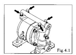
Remove the 4 retainer bolts from the out manifold, and remove the out manifold. [Fig.4.1]
