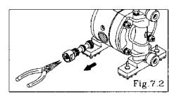
Draw out the C spool valve assembly using the plyer, and remove the seal ring from the C spool valve assembly.
