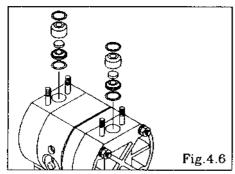
• Remove the O ring, valve stopper, flat valve and valve seat. [Fig.4.6]
