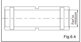
• Throat bearing [Fig.6.4] Measure the inside diameter, and if it is outside the usable range, replace the throat bearing
