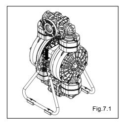
• Remove the 4 cap A and cap B retainer bolts, and remove cap A and cap B. [Fig.7.1]
