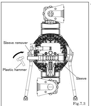
• Remove the sleeve using the sleeve remover (special tool: Part number 713180). [Fig.7.3]
