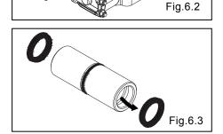
• Remove the packing from the throat bearing. [Fig.6.3]
