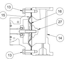
**Diaphragm Orientation** Install diaphragm and spacer as shown above.
