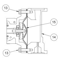
**Diaphragm Orientation** Install diaphragm as shown above.
